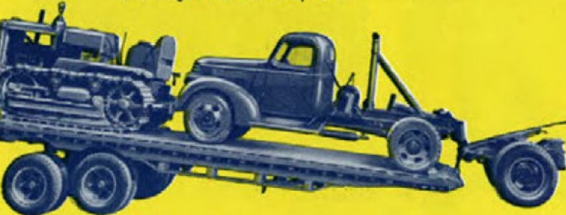
OIL-FIELD FLOAT —a unique flat-bed model for construction and oil-field service. These Trailers are adaptable for loading tractors, bulldozers and self-propelled equipment. Single and Tandem-Axle models of various lengths.
