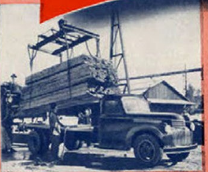
Chevrolet platform trucks, 125 1/4", 134 1/2" and 160" wheelbases (conventionally 109" and 132 1/2" wheelbases (cab-over-engine)—for loads from 2300 to 10,600 pounds.
