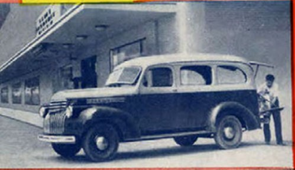
Chevrolet carryall suburban, 115" wheelbase. Removable seats. Ideal for transporting personnel. Accommodates 8 people, instruments and small parts; loads up to 1100 pounds.
