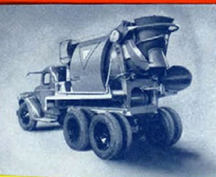
Chevrolet tandem rear axle drive transit concrete mixer, two- to three-yard capacity. Gross allowable up to 30,000 pounds.
