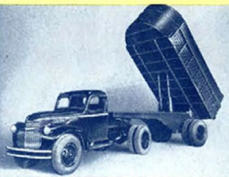
Chevrolet 134 1/2"-wheelbase tractor hauling a semi-trailer dump body with 16-yard capacity.
