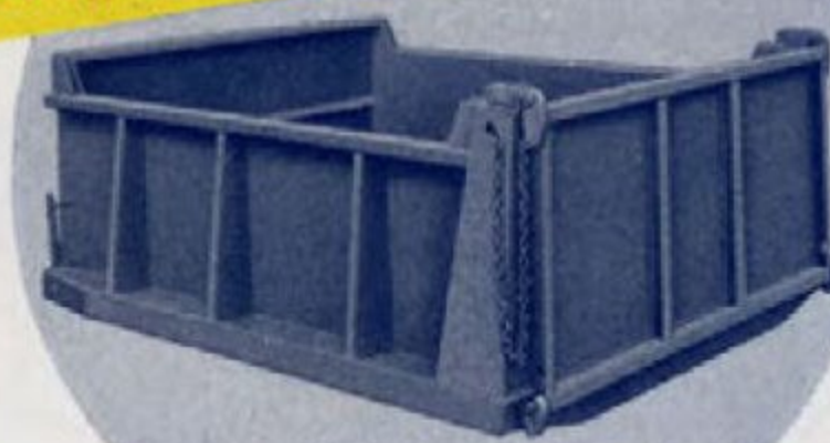
The Heil Contractor's Body has straight sides, square corners, and a double-acting tailgate fitted with offset hinges. V-section side braces provide substantial support and prevent spreading at the tailgate. Sagging body floor is eliminated in all Heil bodies by using both the cross members and long members of the sub-frame for support.
