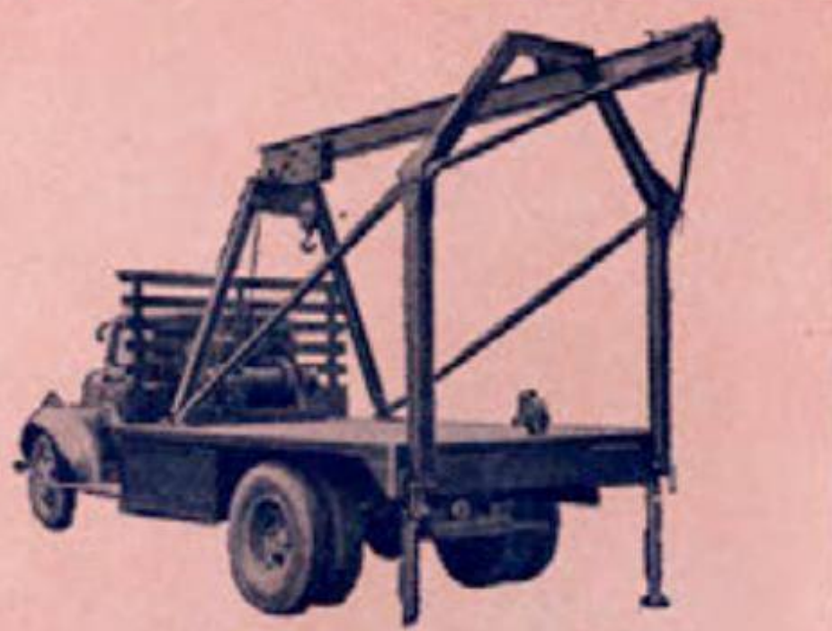
The 2400 Series cranes are equipped with a keyed drum, worm geared winch for power hoisting and lowering, hand winch for boom adjustment, and tag line swing. GAR WOOD Model 2412 (illustrated below).
