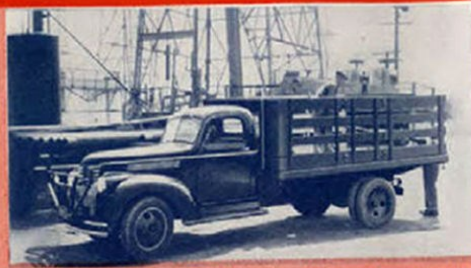
Chevrolet stake trucks, 125 1/4", 134 1/2" and 160" wheelbases (conventionally 109" and 132 1/2" wheelbases (cab-over-engine)—for loads from 2100 to 10,200 pounds
