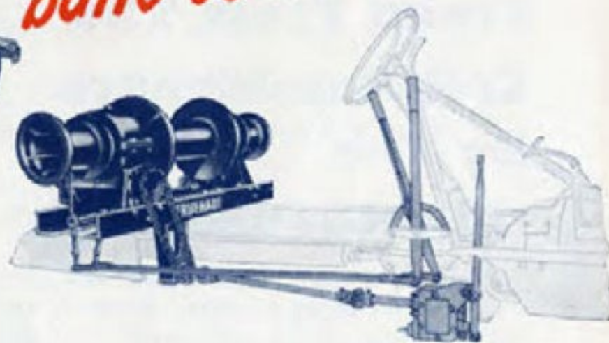
FRUEHAUF WINCHES afford greater safety features such as tapered roller bearings, full automatic safety brake and cast-integral worm gear. 5 capacities — 6,000 lbs. to 25,000 lbs.
