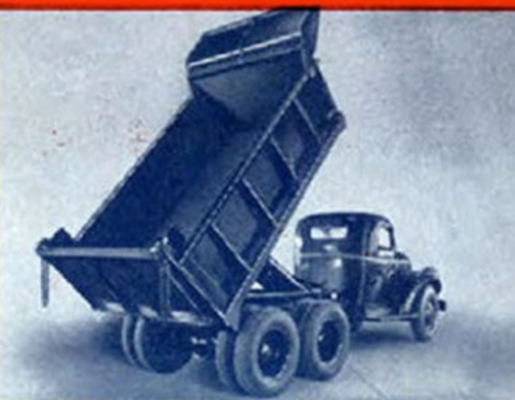
Chevrolet tandem rear axle drive dump truck. Body has six-yard capacity with eight-yard ends.
