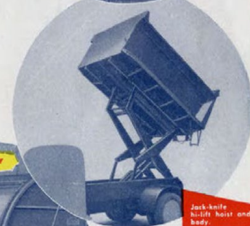
Heil Collecto-pak body provides a quick, efficient, sanitary way of handling garbage.
