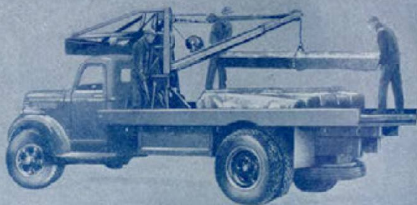
GAR WOOD MODEL Q-D3 (illustrated above). "Quick-Detachable" type. Structural Steel with Tubular Steel Braces. Suitable for 6-ft. tree ball. Effective trolley travel along boom, 11 ft. Hook overhang, 36 in. Crane capacity 3 tons on 2 part line.
